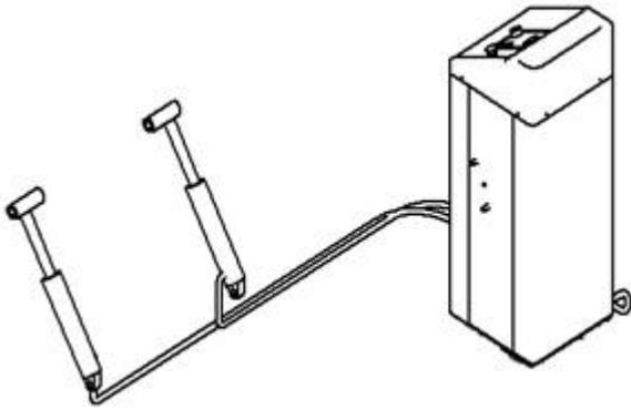
b. Connect the hydraulic assembly with the optional hand pump. Press down the handle of the pump to raise the platforms to have the safety teeth unlocked.
