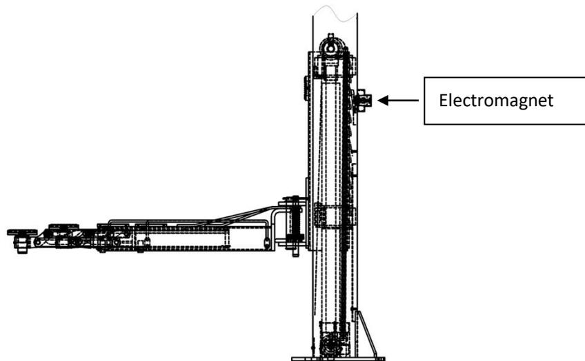
d. Loosen the electrical valve of the power unit to lower the carriage.
