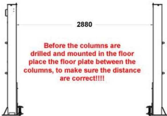
1. It must also be decided on which side the main column should be placed. (Normally left in the access direction is normal)
