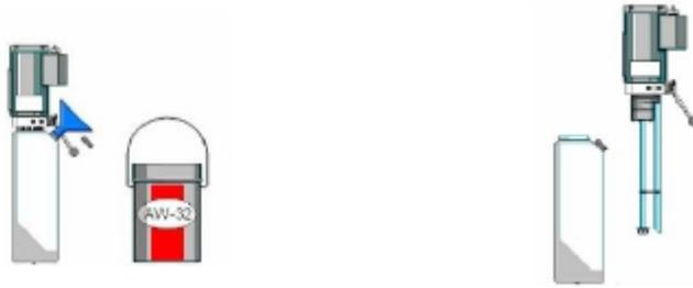
Step 15: When all the steps from 1 to 14 are double-checked, connect the lift to power and try to press the "UP" button (Do not place any vehicle in this step)
