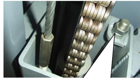
The bolt and nut to adjust the calibration wire
