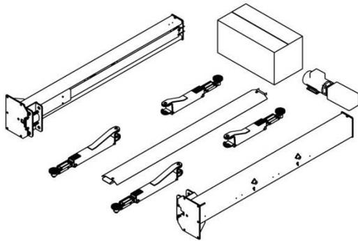
Step 5: Decide the installation position of the columns, erect the main and assistant post. Pay attention that the width between posts is 2880m.
