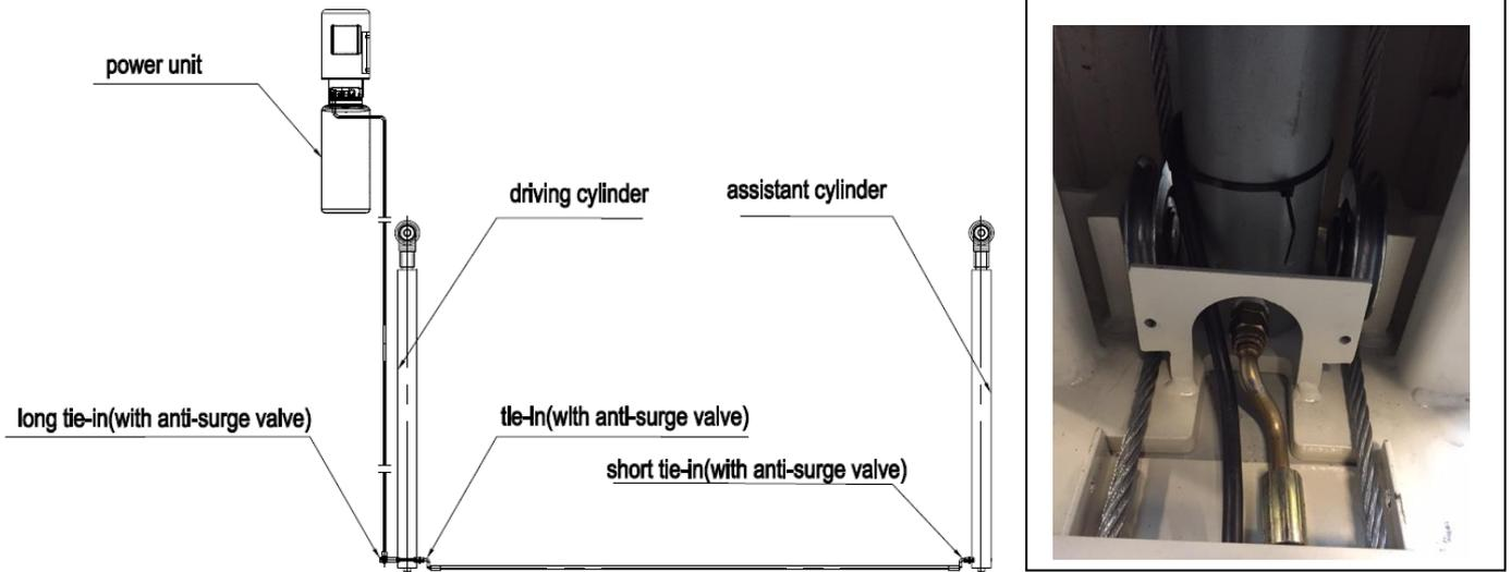
Step 10: Install four safety plates, four electromagnets and the electromagnet covers. Connect the wire to electromagnets.
